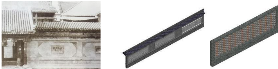
Fig 77. Partitions designed in the form of external walls of traditional residential courtyards
