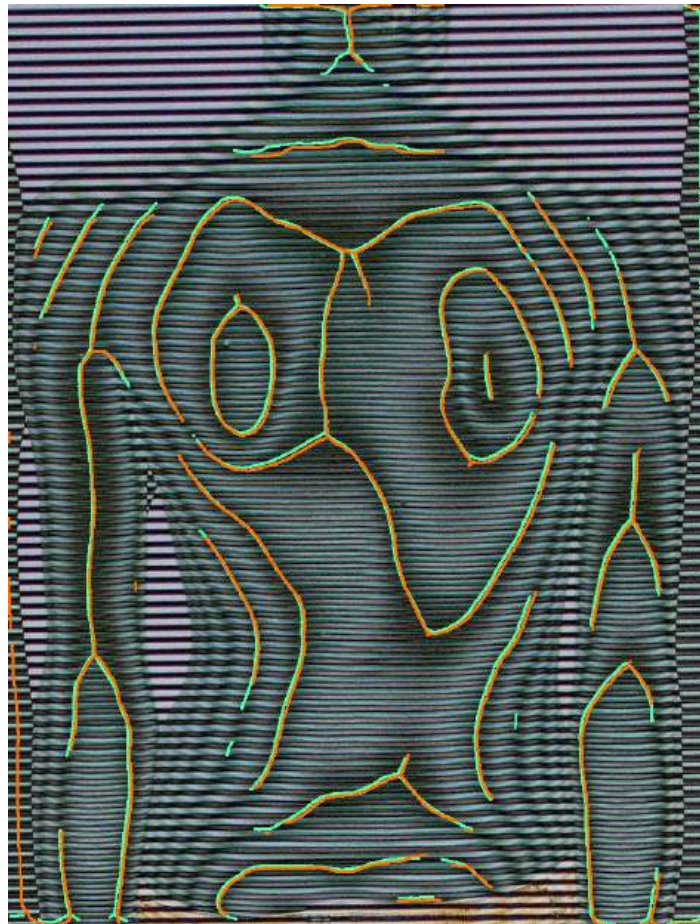
Fig. 51: Static (orange) and adaptive (green) segmented moiré fringes on image no. 4
