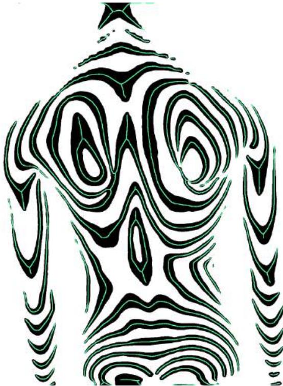
Fig. 42: Overlay of adaptive segmented moiré fringes (green) on thresholded image (black)
