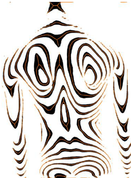
Fig. 34: Overlay of segmented moiré fringes (orange) on thresholded image (black)
