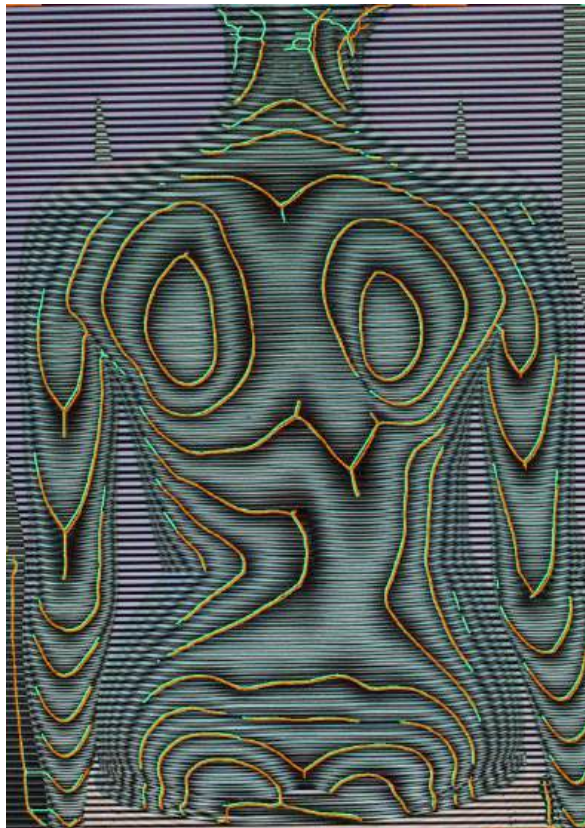
Fig. 49: Static (orange) and adaptive (green) segmented moiré fringes on image no. 3.
