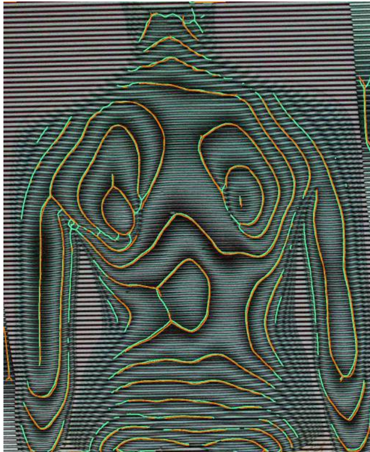
Fig. 53: Static (orange) and adaptive (green) segmented moiré fringes on image no. 5.
