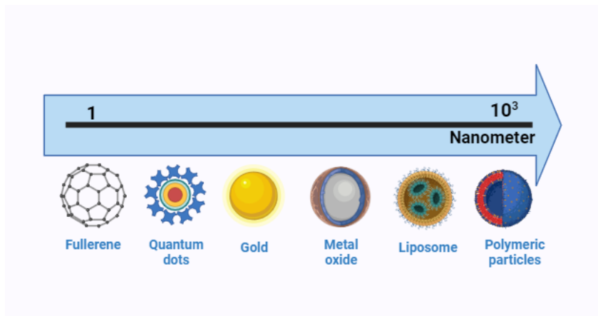
Figure 1.1: Illustration representing different types of spherical nanoparticles across a size spectrum spanning from 1 to 1000 nanometers. ( Illustration edited using BioRender )
