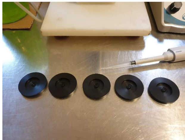
Figure 12: Calibration disk with 100µl algae suspension for cross-check
