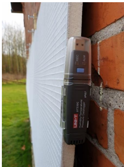
Figure 15: Position of data recorder at the test panel
