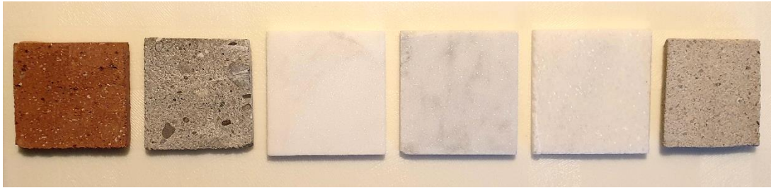
Figure 8: Material samples (from left to right: brick, concrete, marble fine, marble grey, marble coarse, lime-sandstone)
