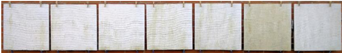
Figure 19: Biofilm visual impression of weathered samples after 730 days
