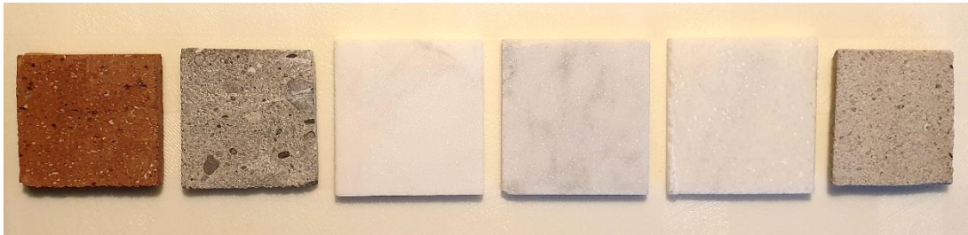
Figure 29: Material samples (from left to right: brick, concrete, marble fine, marble grey, marble coarse, lime-sandstone)
