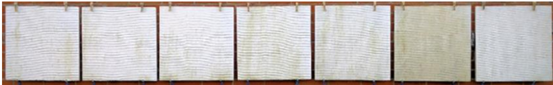
Figure 56: Biofilm visual impression of weathered samples after 730 days
