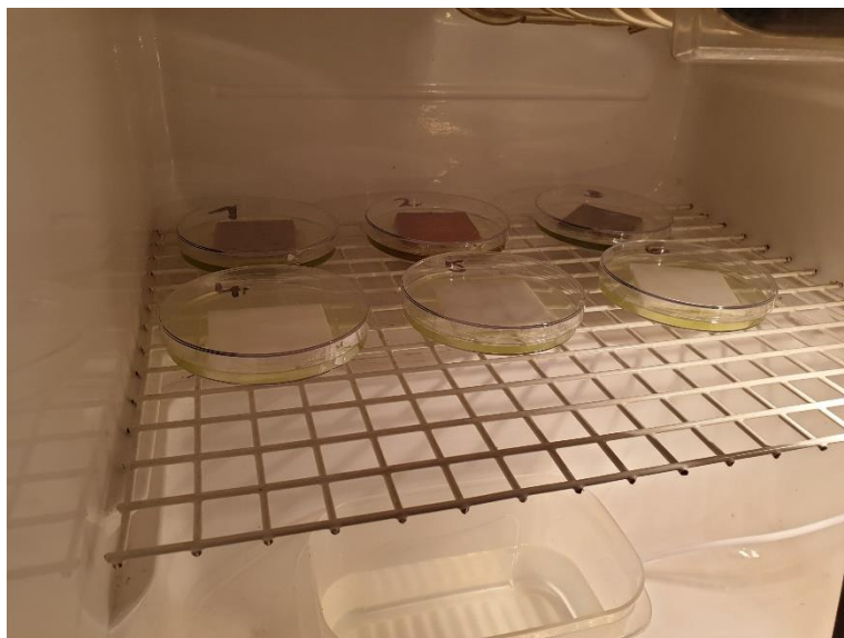
Figure 30: Incubation chamber with cultivation lamp and samples
