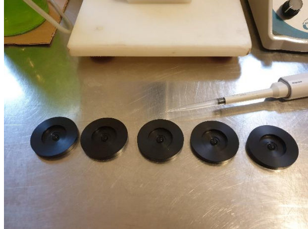
Figure 42: Calibration disk with 100µl algae suspension for cross-check
