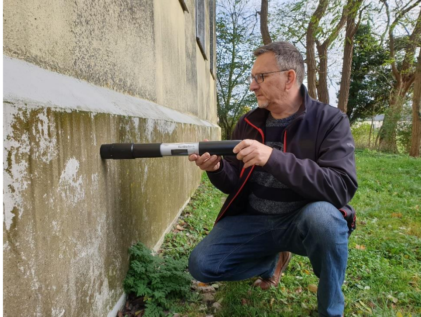
Figure 3: Biofilm detection with BenthoTorch® at Görslow Church 2020
