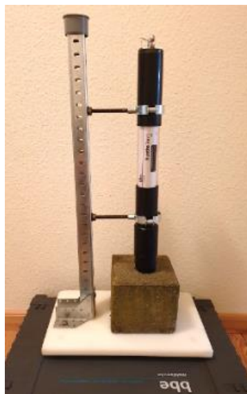
Figure 19: Tripod construction stand for interval measurements
