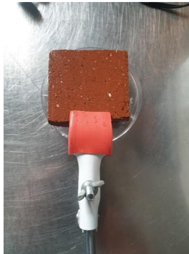
Figure 41: Clamp as immersing tool for suspension test
