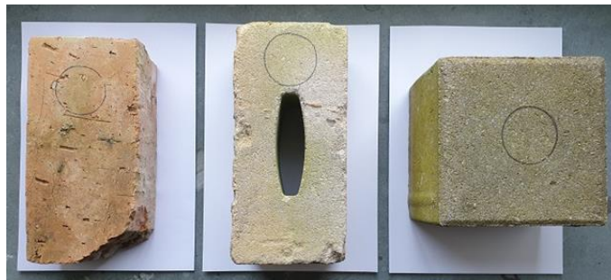
Figure 18: Material samples after 3 years of weathering (brick, lime sandstone, concrete)
