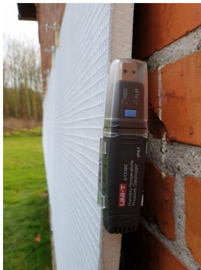
Figure 49: Position of data recorder at the test panel
