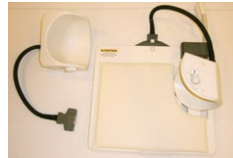
Figure I.28. Dedicated phase array shoulder coils
