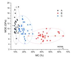
Figure 3. MOE vs. MC 95% confidence ellipse graphs for the three groups of tested samples
