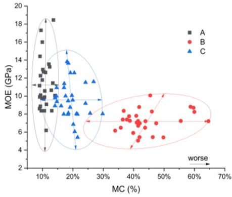
Figure 3. MOE vs. MC 95% confidence ellipse graphs for the three groups of tested samples
