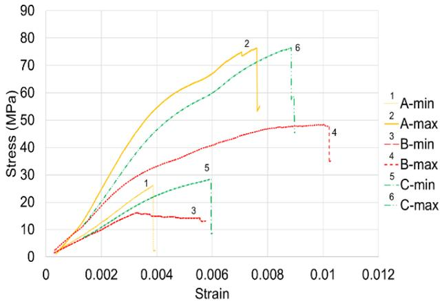
*Figure 1. Stress vs. strain diagram for maximum and minimum strength of rupture of tested groups*
