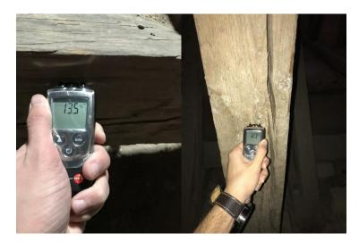
Figure 20. Moisture content measurements in the timber elements of the roof
