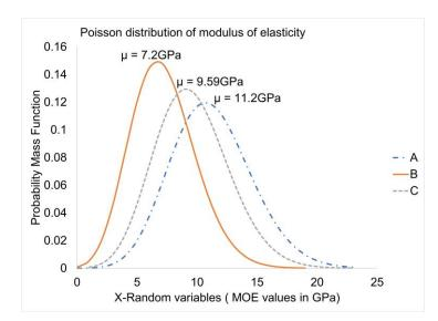
Figure 61. Modulus of elasticity representation in terms of Poisson's distribution
