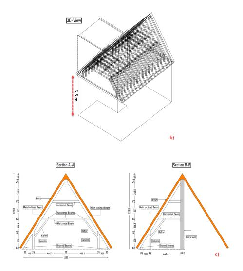
Figure 18. Roof sketch based on the visual inspection: a) plan view; b)3D view; c) section view
