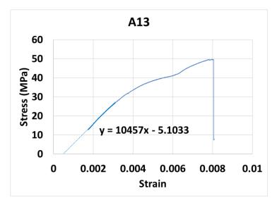
Figure 50. Stress vs. strain diagram for sample A13
