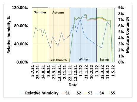
Figure 39. Stairs moisture content and relative humidity vs. date (Makovecz Imre tower)
