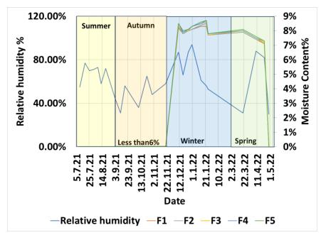
*Figure 41. Fences moisture content and relative humidity vs. date (Makovecz Imre tower)*
