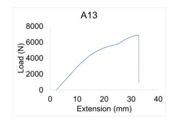
Figure 48. Load vs. displacement curve generated by the testing machine for sample A13
