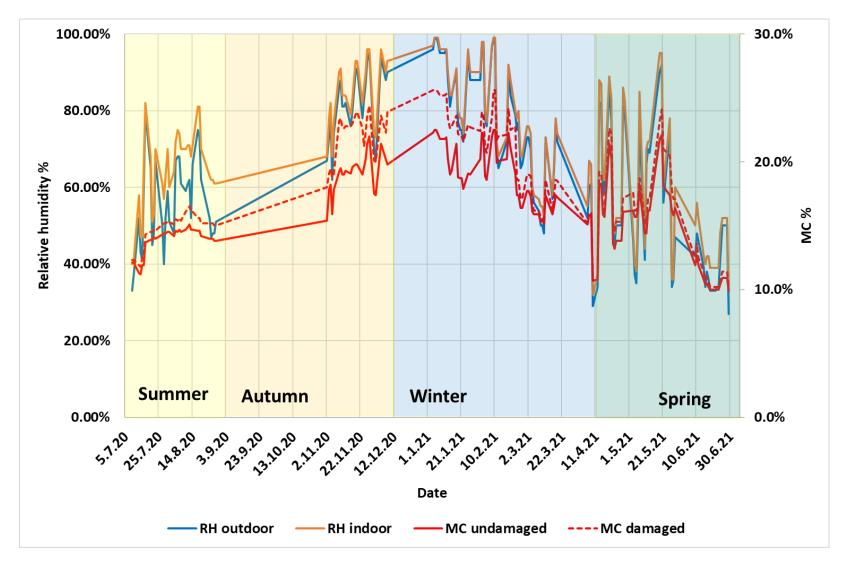
Figure 26. Columns moisture content and relative humidity vs. date
