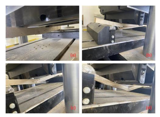
Figure 52. Failure modes found during the test for the case of group A, a) simple tension failure; b) crossgrained tension failure; c) brash tension failure; d) buckling failure
