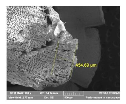
Figure 64: Protecting layer penetration depth in SEM measurements
