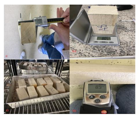
Figure 51. a) geometry measurements b) weight measurements c) drying samples d) surface MC measurement
