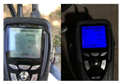
Figure 21. Devices for the outdoor and indoor measurements of temperature and relative humidity
