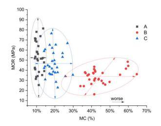
Figure 57. MOR vs. MC - 95% confidence ellipse graphs for the three groups of tested samples
