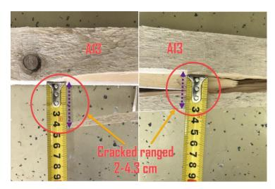
Figure 54. Crack width measurements for A13
