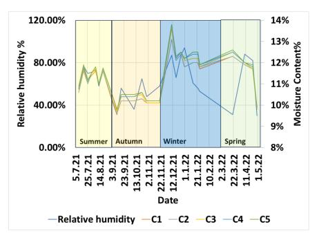
Figure 37. Columns moisture content and relative humidity vs. date (Makovecz Imre tower)
