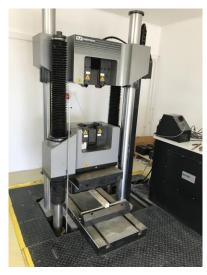
Figure 13. Instron static hydraulic machine - Satec series [own photo]
