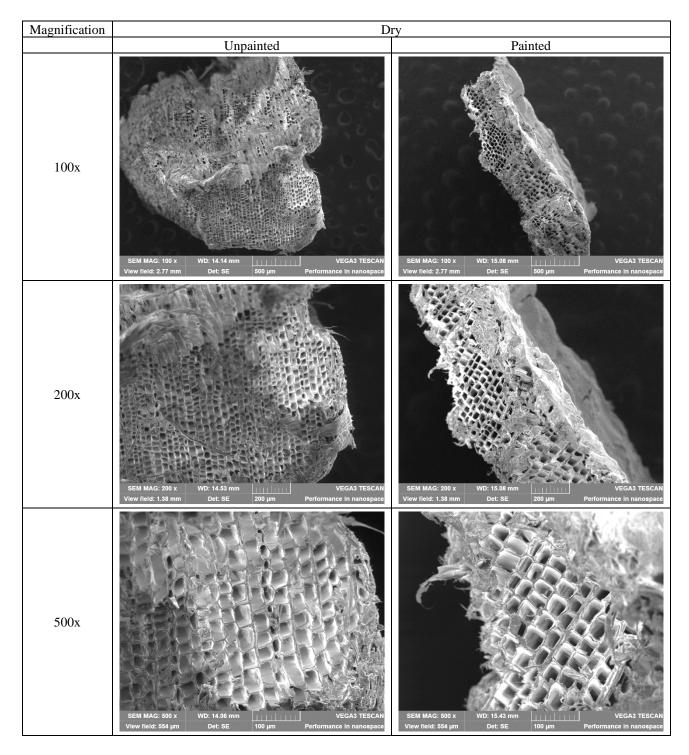
Table 12: Examples of SEM measurements on Picea Abies samples
