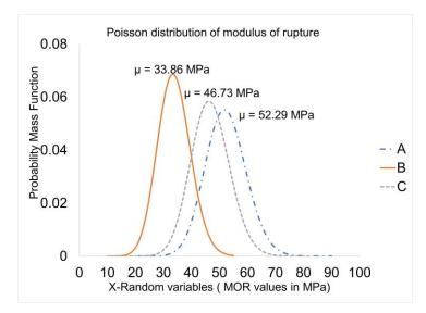
Figure 60: Modulus of rupture representation in terms of Poisson's distribution
