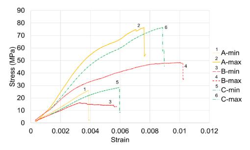
Figure 53. Stress vs. strain diagram for maximum and minimum strength of rupture for the tested groups
