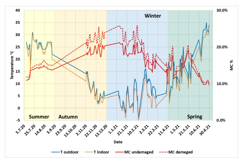
Figure 24. Rafters moisture content and temperature vs. date
