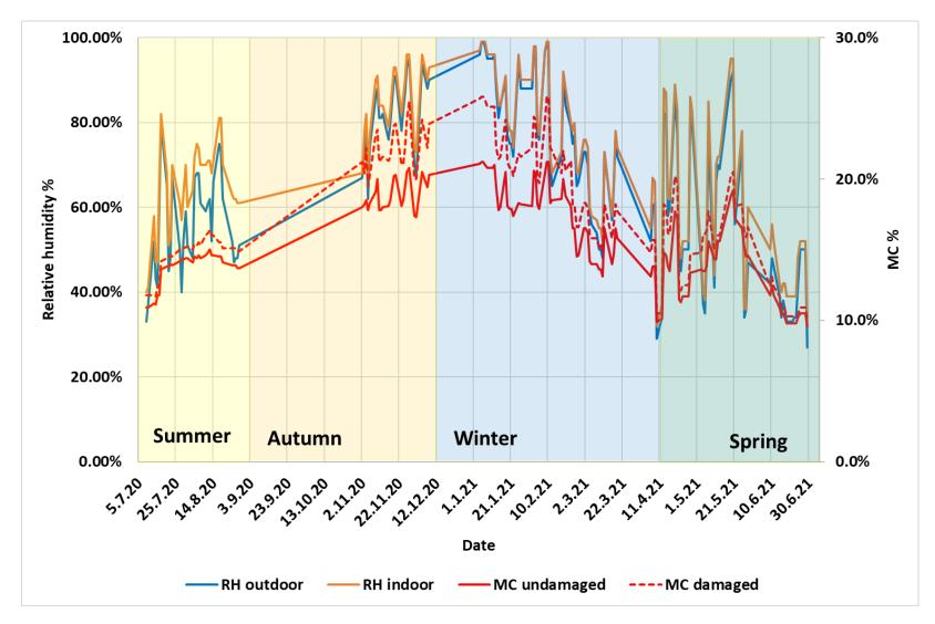
Figure 27. Rafters moisture content and relative humidity vs. date
