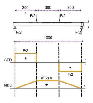
Figure 47. Load analysis of the testing sample
