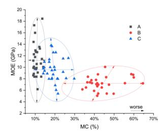
Figure 58. MOE vs. MC - 95% confidence ellipse graphs for the three groups of tested samples
