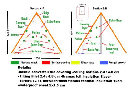
Figure 19. Positions of cracks and defects found in the roof of Civil Community House
