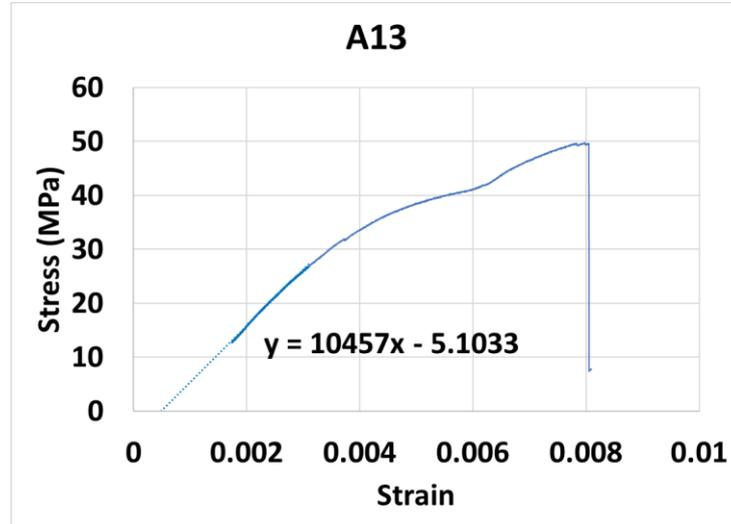
Figure 50. Stress vs. strain diagram for sample A13
