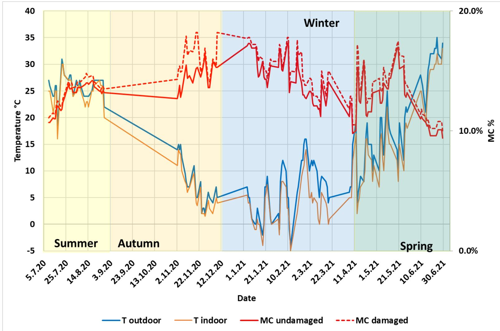
Figure 22. Beams moisture content and temperature vs. date
