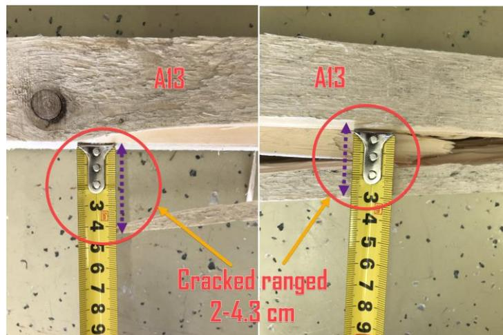
Figure 54. Crack width measurements for A13
