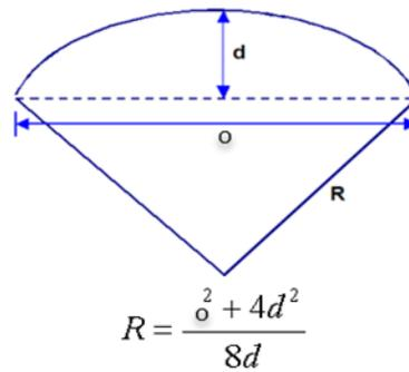
Figure 49. Radius of curvature
