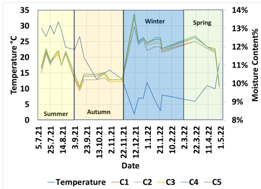
Figure 36. Columns moisture content and temperature vs. date (Makovecz Imre tower)
