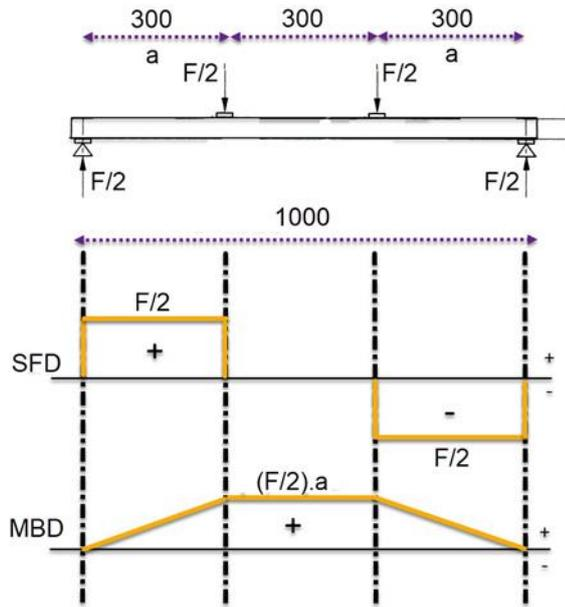
Figure 47. Load analysis of the testing sample
