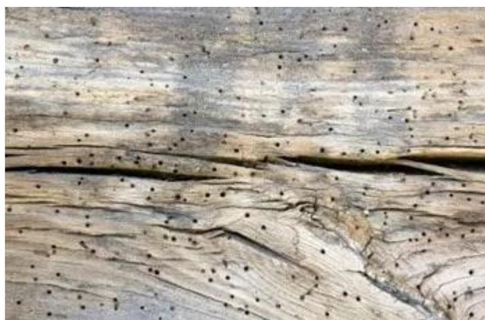
*Figure 2. Beetles defects in timber [The Constructor, 2021]*
