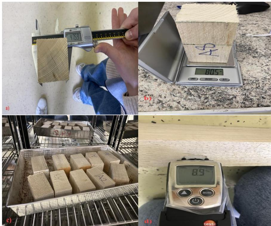
Figure 51. a) geometry measurements b) weight measurements c) drying samples d) surface MC measurement
