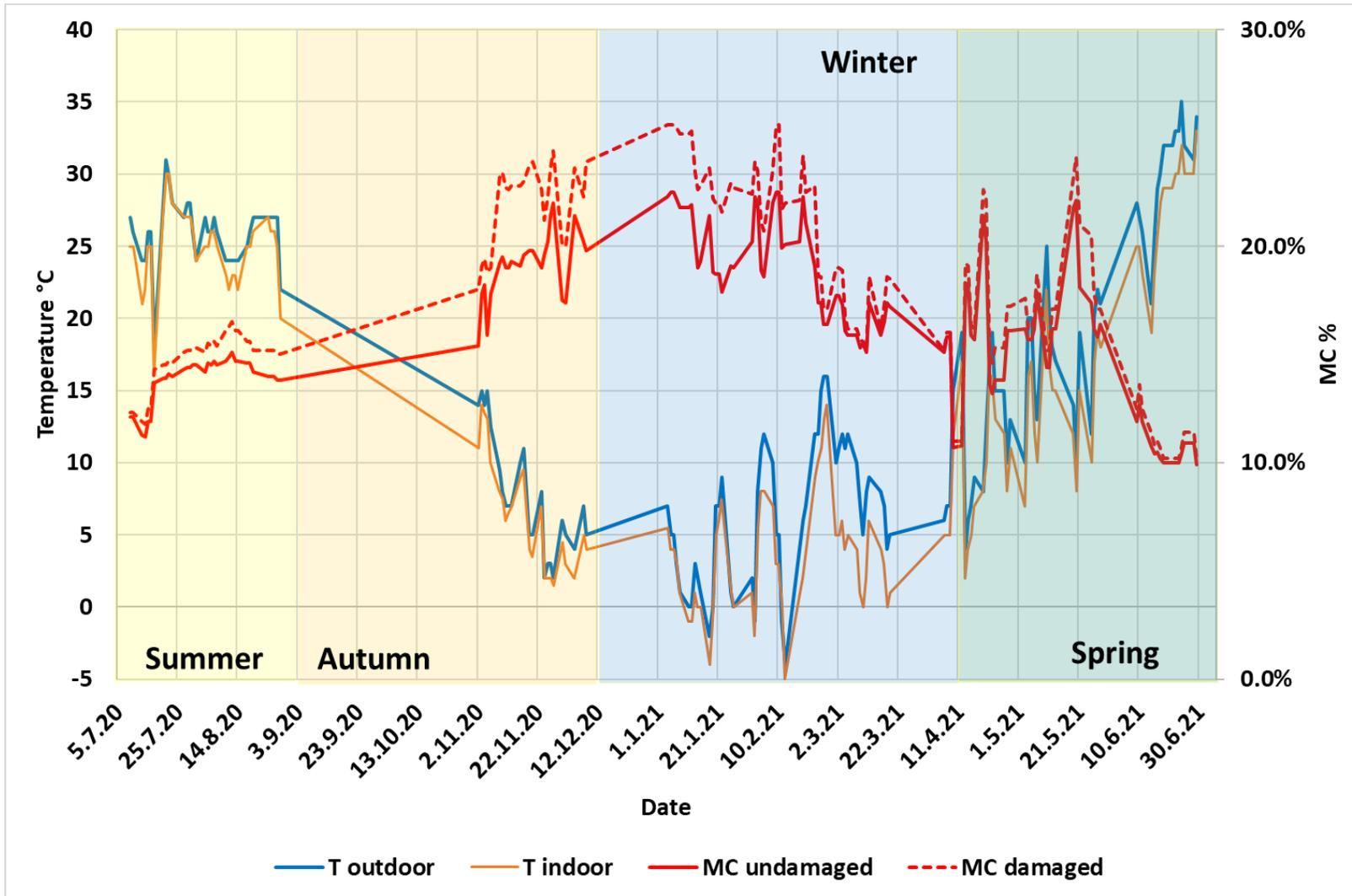
Figure 23. Columns moisture content and temperature vs. date
