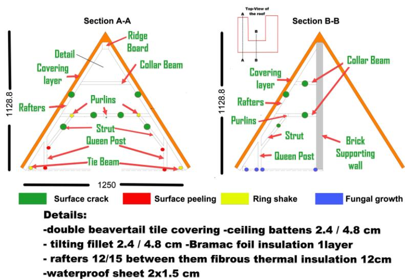
Figure 19. Positions of cracks and defects found in the roof of Civil Community House
