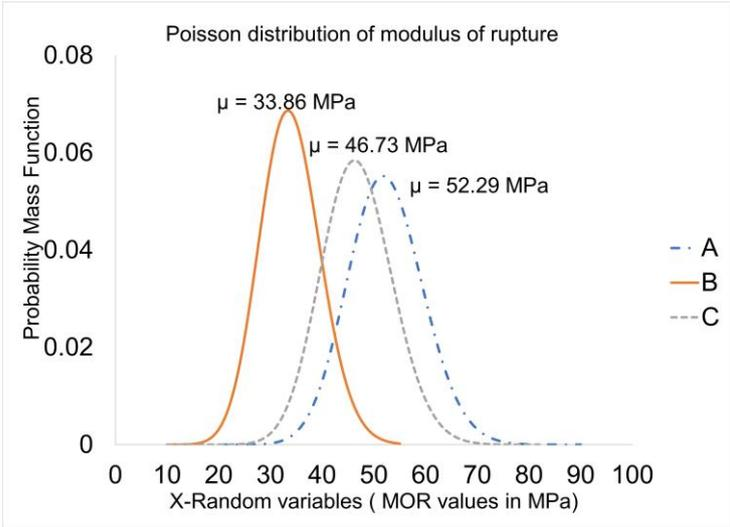
Figure 60: Modulus of rupture representation in terms of Poisson's distribution
