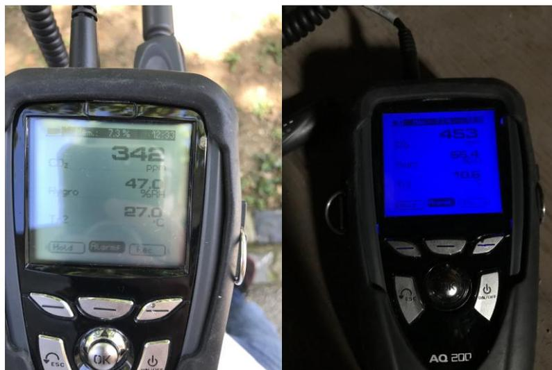
Figure 21. Devices for the outdoor and indoor measurements of temperature and relative humidity
