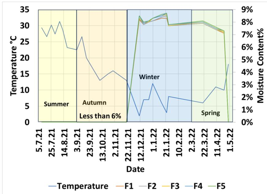
Figure 40. Fences moisture content and temperature vs. date (Makovecz Imre tower)
