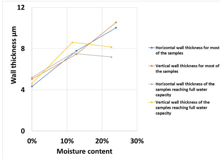
Figure 63. SEM results, MC vs. wall thickness
