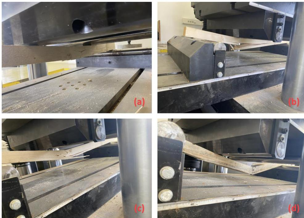
Figure 52. Failure modes found during the test for the case of group A, a) simple tension failure; b) cross-grained tension failure; c) brash tension failure; d) buckling failure
