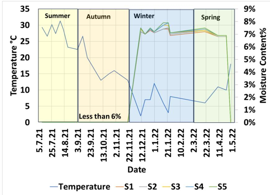
Figure 38. Stairs moisture content and temperature vs. date (Makovecz Imre tower)
