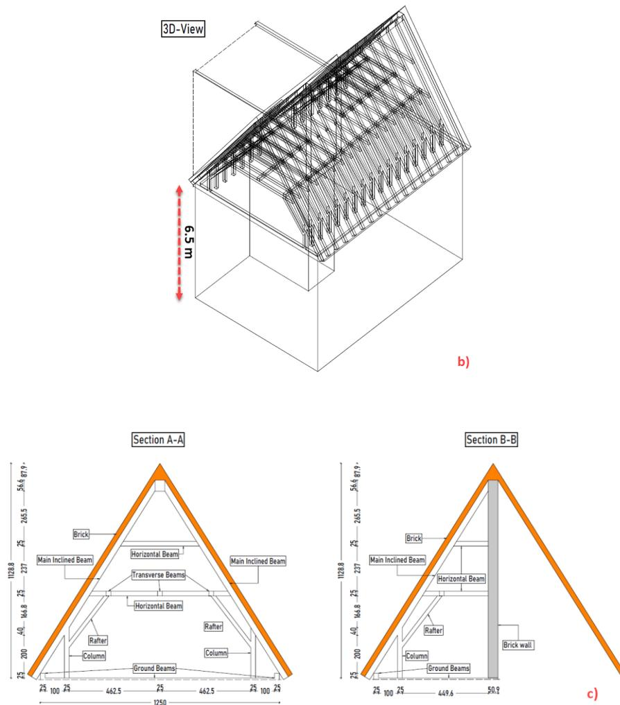
Figure 18. Roof sketch based on the visual inspection: a) plan view; b) 3D view; c) section view
