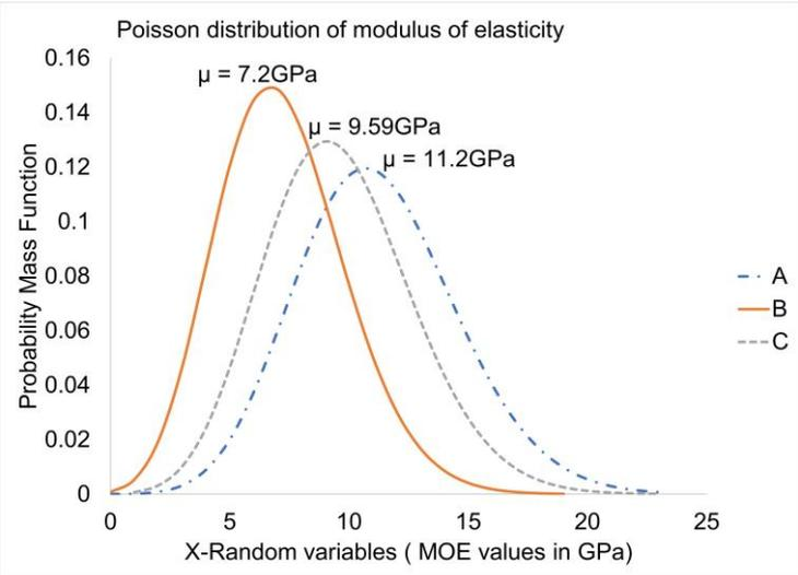
Figure 61. Modulus of elasticity representation in terms of Poisson's distribution
