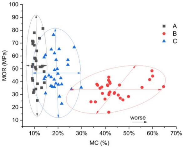
Figure 57. MOR vs. MC - 95% confidence ellipse graphs for the three groups of tested samples
