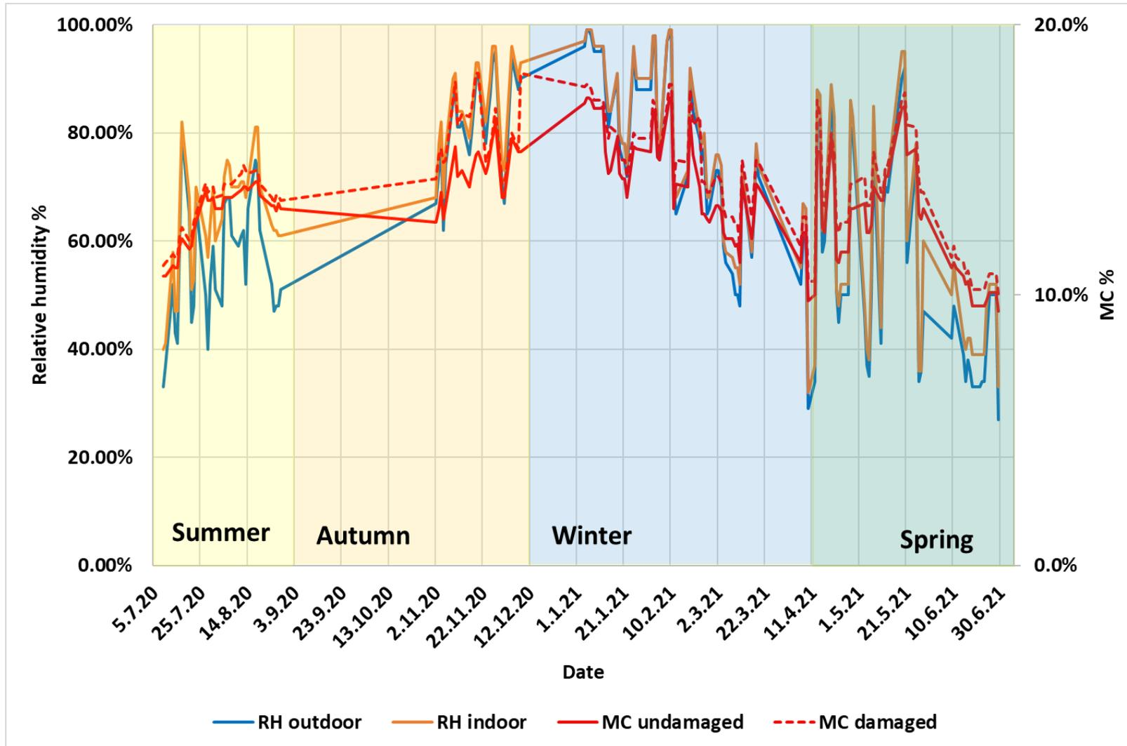
Figure 25. Beams moisture content and relative humidity vs. date
