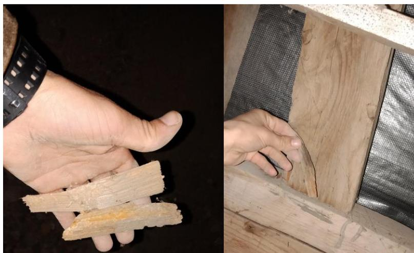
*Figure 62. Collected samples for SEM*
