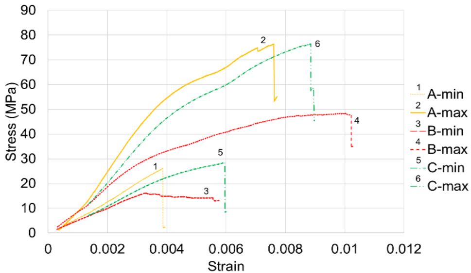
Figure 53. Stress vs. strain diagram for maximum and minimum strength of rupture for the tested groups
