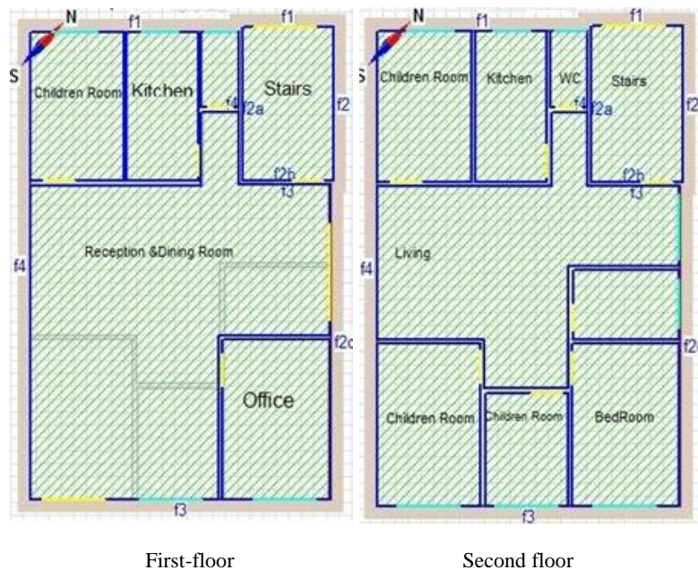
Figure 4-1. Building zones for the first and second-floor plan of the dwelling object of study.
