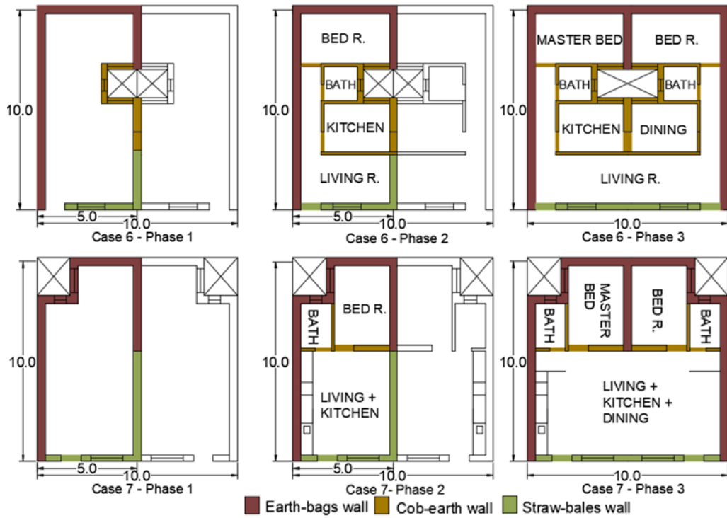
Figure 5-5 Compact vertical sited plot layout design Cases (Cases 6 and 7) with their three phases
