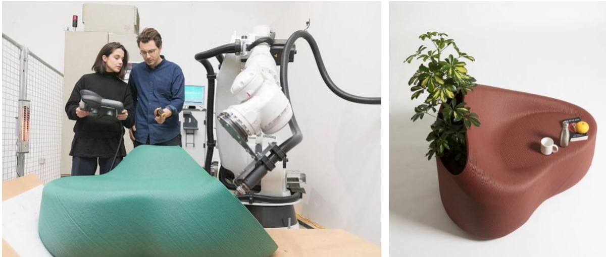
Figure 58. a-b 3D printer in serve of transforming plastic into urban street furniture
