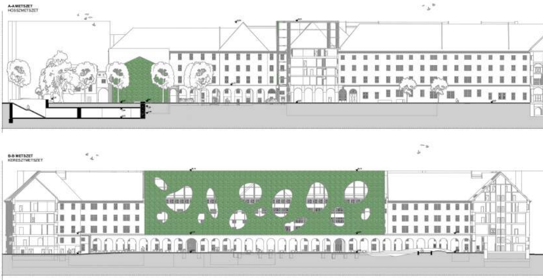
Figure 153, 154: Green facade at the town hall facade and the living wall at Merlin theatre facade, technique drawing by the design team
