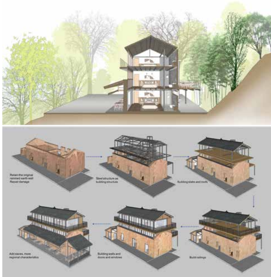
Fig 5.14: Sectional view and generated exploded view of Building 1(source: drawing by author )
