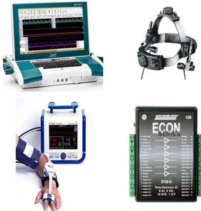
Figure 11. Hardware used to detect physiological changes in blood pressure and intracranial blood flow velocity indicating functioning neurovascular coupling. Top left: Blood flow velocity (FV) was detected by a transcranial Doppler ultrasound device (Multi-Dop T, Compumedics DWL, Singen, Germany). Top right: A head frame was used to steady the TCD's transducers at correct positions in order to continuously measure blood flow in both middle cerebral arteries. Bottom left: A non-invasive finger cuff monitor (CNAP® Monitor 500 HD, CNSystems, Graz, Austria), to record beat-to-beat blood pressure continuously based on blood volume changes in the finger (plethysmography). Bottom right: Analogous BP and FV signals are converted to digital signals and forwarded to a computer by a data acquisition (DAQ) A/D converter device (DT9816, Measurement Computing Corporation, Norton, MA, USA)
