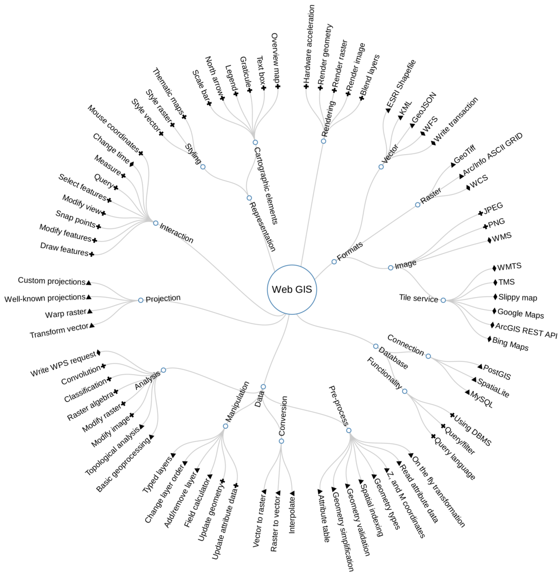
Figure 5: Features of a basic universal massive Web GIS client grouped by functionality. Triangles, crosses, and diamonds denote GIS-specific features, non-GIS-specific features, and web mapping specific features respectively (Farkas, 2017a).
