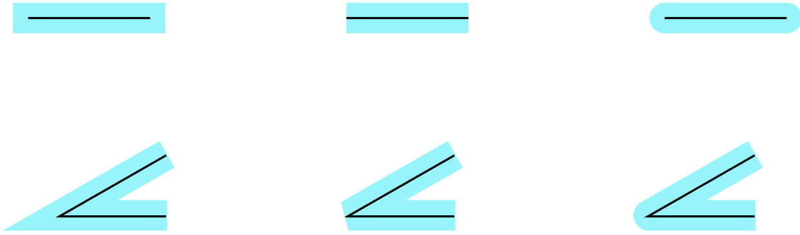
Figure 16: Relationship of base lines (black) with their respective line caps (top row) and line joins (bottom row). Line caps can be square (left), butt (center), and round (right). Line joins can be miter (left), bevel (center), and round (right).
