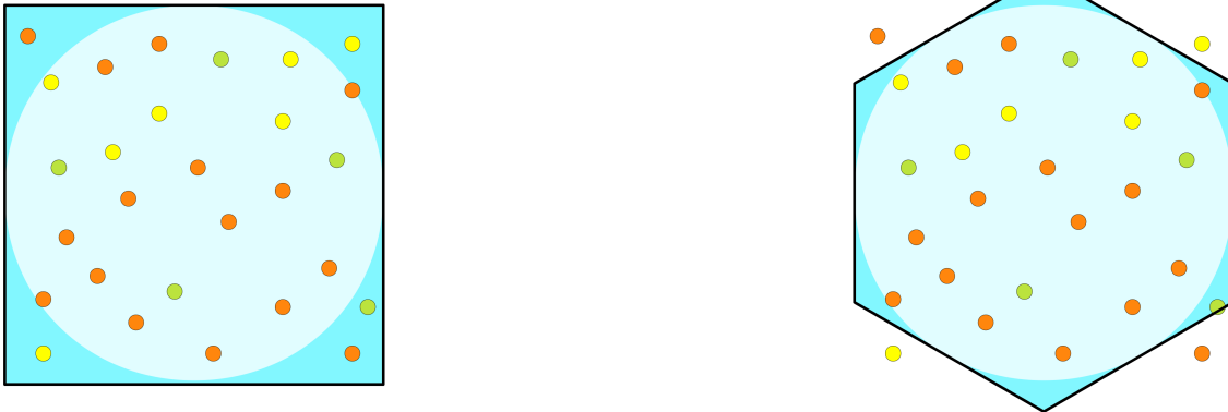
Figure 26: Sampling bias with a square, and a hexagonal cell. Observations in lighter areas (inscribed circles) can be aggregated without concerns, since they equally represent the center of the cell. Observations in darker areas, however, are contributing to the overall bias of sampling.
