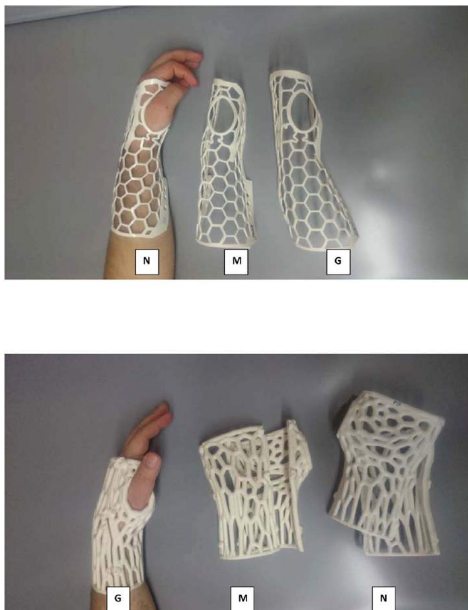
Figure 6. (a) Thermoformed models of wrist splints. N: neat PLA, G: Gypsum PLA, M: Modell PLA. (b) 3D scanned models of wrist splints. N: neat PLA, G: Gypsum PLA, M: Modell PLA.
