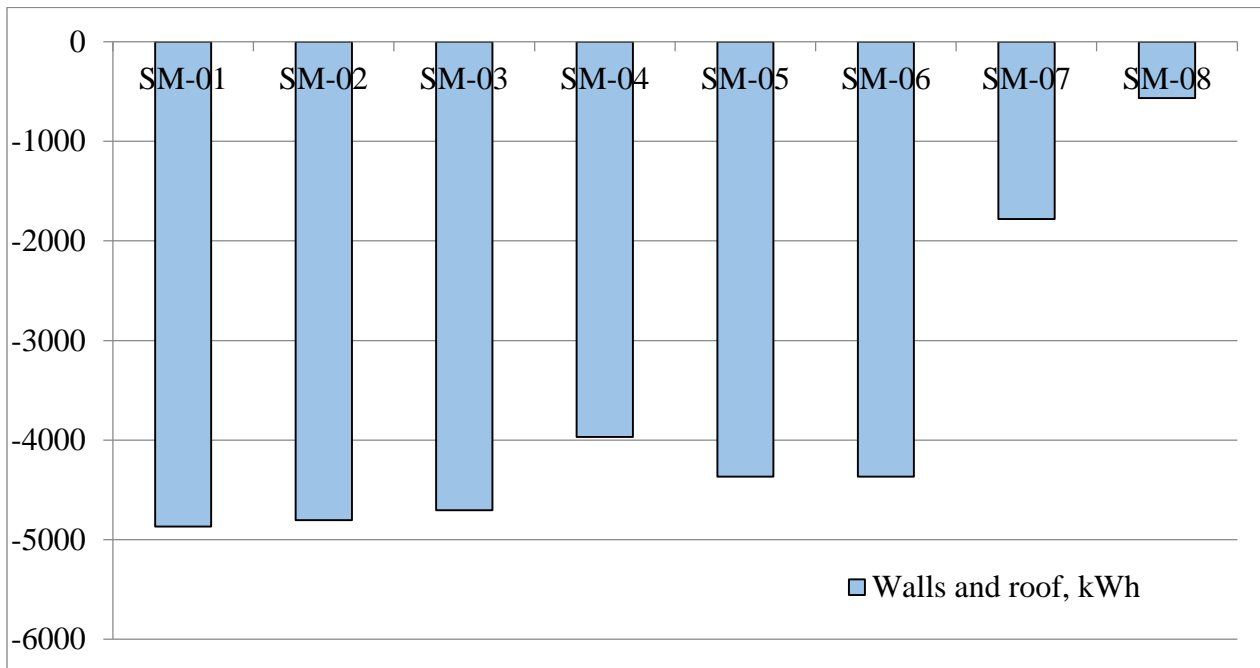
Figure 61: Heat loss from the details of a yurt in heat balance
