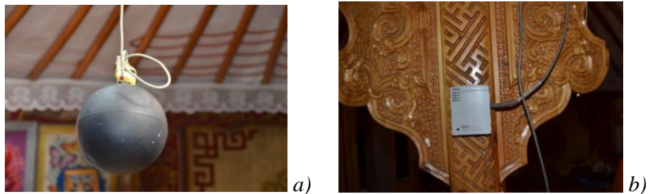
Figure 25: Measurement tools for the yurt a) Radiation temperature measurement, b) Air temperature measurement (HOBO)
