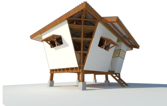
Figure 1. Slanted Exterior Walls of the Shelter and corner wall (exposed)
