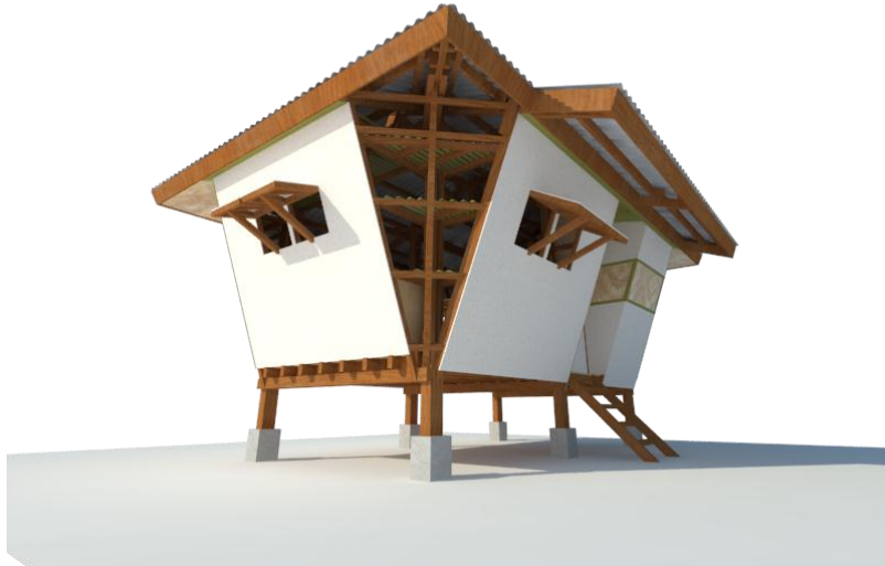
Figure 41. Slanted Exterior Walls of the Shelter and corner wall (exposed)
