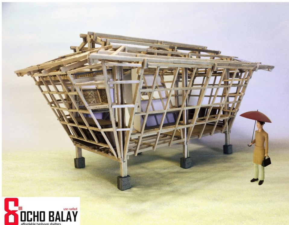
Figure 78. Scale model of the Ocho Balay Typhoon Shelter. The structural framings are shown here in detail.
