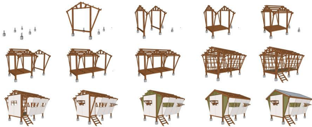
Figure 29. The construction process of the shelter.
