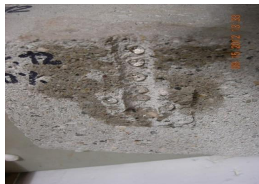
Fig. 4: Remaining droplets on the surface due to hydrophobicity after application of the IM
