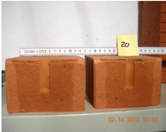
Fig. 5: Failure plan of the sample after splitting. The darker areas are due to the spreading of the IM
