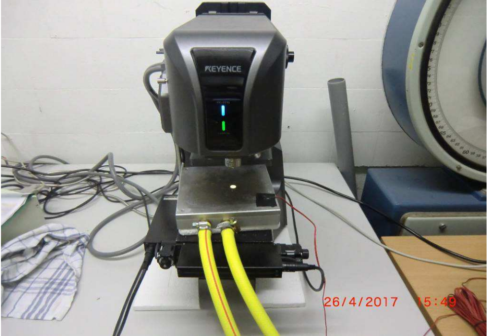
Fig. 08: Experimental set-up with Keyence VK 9700 laser scanning microscope and cooling plate.
