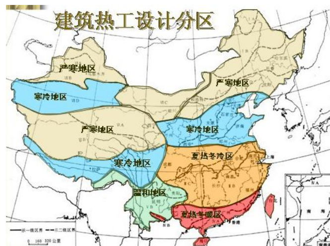
Fig. 2.2 China Construction Thermal Division Map
