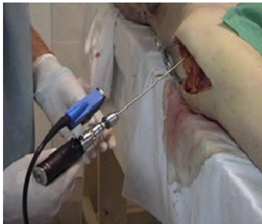
Figure 12.7 EM sensor mounted and calibrated to the navigated Synthes pneumatic drill.
