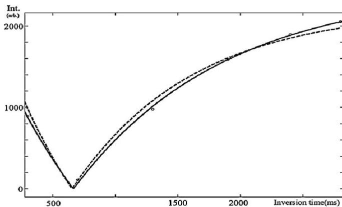
**Figure 7: Comparison of two- and three-parameter fits used for  $T1$  measurement.** The equations for the fits are presented in the Methods section. The intensity (arbitrary units) obtained from a rat cortex is plotted against the inversion time (ms). Dashed and continuous lines correspond to the two- and threeparameter fits, respectively.
