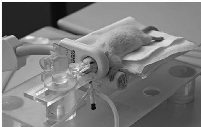
*Figure 3: The custom-built head holder with the 40mm (i.d.) loop coil. The rat is intubated and anesthetized.*
