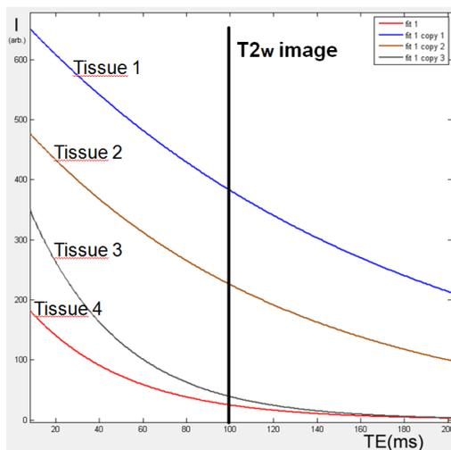
Figure 1. Quantitative vs. Qualitative imaging This figure shows the T2 relaxation time curves obtained from quantitative measurements of 4 different tissues. The quantitative data describes the signal intensity during the whole T2 relaxation process.
