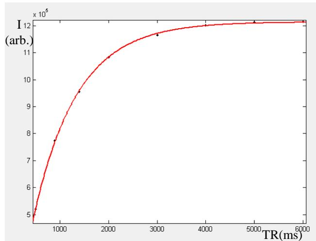
Figure 2: T1 relaxometry is performed in a way of analyzing a series of T1w qualitative images differing only in the repetition time. The measured MR signal of a sample is presented by different repetition times. By fitting a curve on the intensities a quantitative parameter of T1 time can be calculated.
