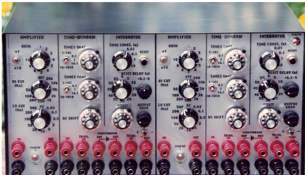
Fig. 6. Photograph of a two-channel evoked response analysis system (built by Sándor Farkas), each channel comprising a signal conditioning amplifier, a time-window unit and an integrator.
