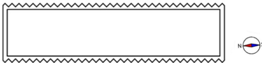
Figure 9. Double-skin façade Zig-zag design
