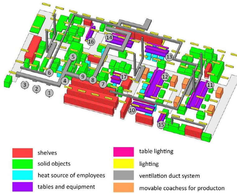
Figure 8. Internal heat gains from occupants, equipment and artificial lighting in the production hall.
