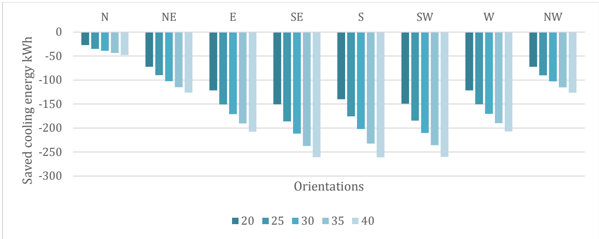
Figure 57. The cooling demand after the application TG
