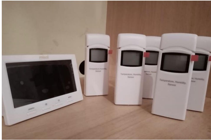
Figure 16. Data logger used for the Measurements collection (Author)
