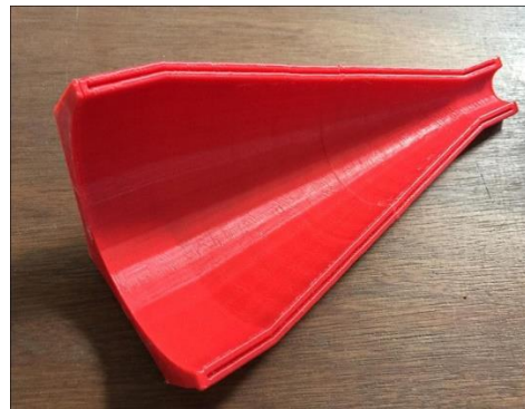
Image 2. A 3D printed Cross section of a Wind Boy with an option for liquid cooling.
