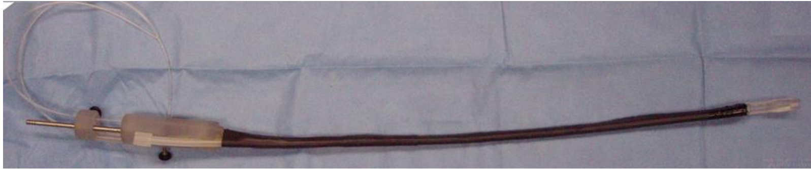
Figure 20. The working prototype of the Barrett's excision device with a flexible shaft, excision capsule and multifunctional handle.
