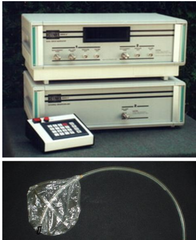
Figure 8. The Barostat and its catheter with the flaccid bag. After calibration of the Barostat, a balloon catheter was delivered and positioned endoscopically in the GEJ. Volumes of the GEJ at pressures from 3 to 21 mmHg in six steps were recorded. After completion the catheter was withdrawn.
