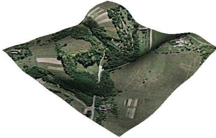
Figure 9. A satellite photo mapped as a texture onto the NURBS surface (Edited by P. BOYTCHEV)
